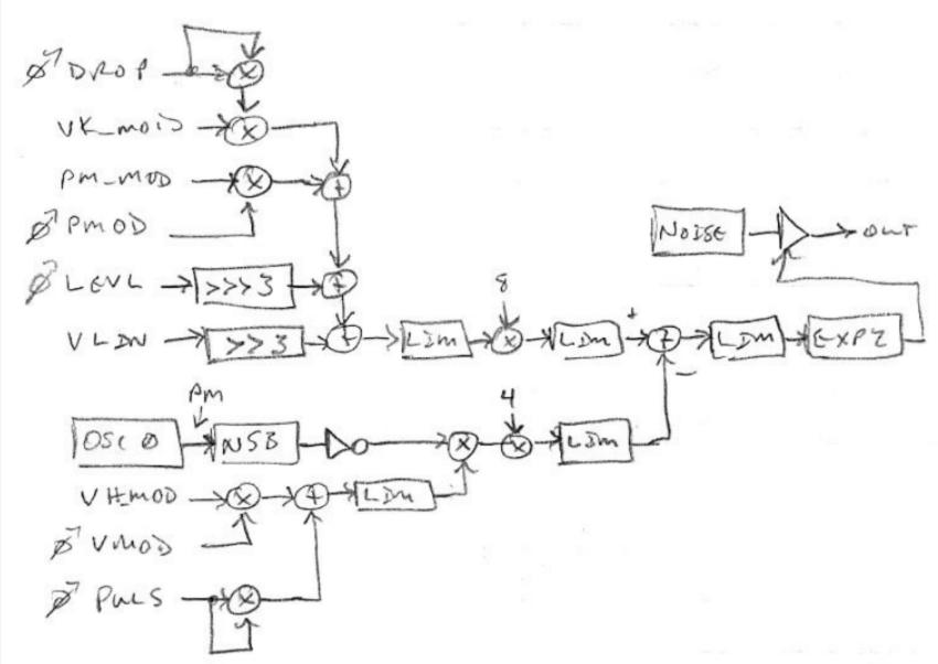
Above is the current noise modulation scheme. The upper main section simply modulates the overall noise envelope with the volume and pitch axes. The lower section is new, and uses the PM process just discussed. We modulate the flipped PM signal with a knob that sets the static PM gain, and vary this with the volume axis number. This is subtracted from the noise level, exponentiated, and used to finally modulate the noise level.
