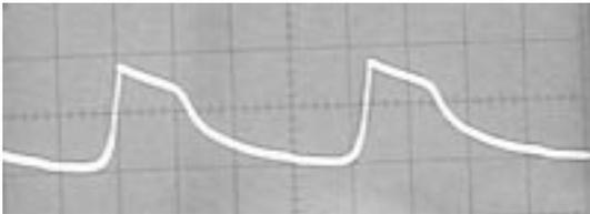
The use of the **MPSA42-AP** transistor has special qualities discovered by experimentation. In theremin design to get a more natural sound my thought was let’s make the RF section more sluggish, this idea comes from my vacuum tube design in how it had a **better droop** at the bottom of the wave shape. The skew on top is the even harmonics.
